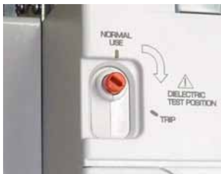
SELECTOR SWITCH IN "TRIP" POSITION: The selector switch is in the extended position, the voltage taps are disconnected from the power supply. It is impossible to close the DMX 3 , and if it was in the closed position, its poles are still open. Dielectric tests can be performed.
