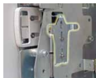
The "Z" parts of both devices should be installed for translational motion, as in the photo
