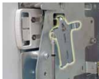
The "Z" parts of all three devices should be installed for rotation, as in the photo
