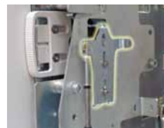
The "Z" parts of all three devices should be installed for translational motion, as in the photo
