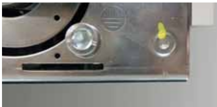
Connection point on the fixed DMX 3
