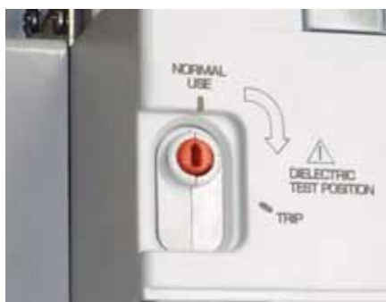
SELECTOR SWITCH IN "NORMAL USE" POSITION: The selector switch is pressed and the voltage taps of the protection unit are connected to the power poles. The DMX 3 can be used normally.
