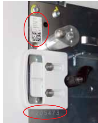
On the right side of the DMX 3 , the end of the serial number is engraved on the metal structure and is shown in full, with the date of manufacture on a sticker.
