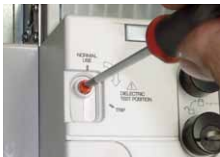
SELECTOR SWITCH IN "TRIP" POSITION: The selector switch is in the extended position, the voltage taps are disconnected from the power supply. It is impossible to close the DMX 3 , and if it was in the closed position, its poles are still open. Dielectric tests can be performed.
