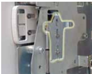
The "Z" parts of all three devices should be installed for translational motion, as in the photo
