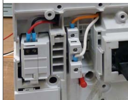
Remove the upstream and downstream rear blanking plates.
