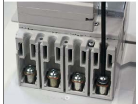
Tighten the upstream and downstream electrical connections using the eight (or six) screws supplied with the circuit breaker. Apply a tightening torque of 7 N·m.
