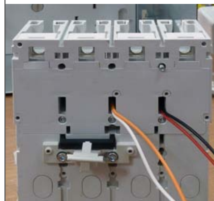
Remove the upstream and downstream cage terminals.
