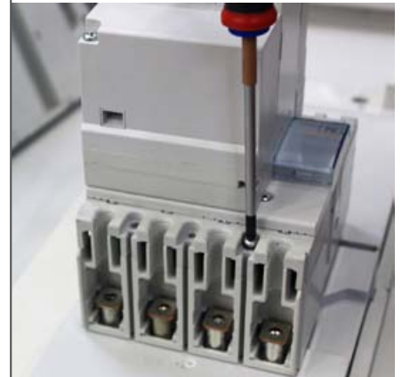
Place the appliance on the base, then secure it with the screws supplied with the circuit breaker (tightening torque 1 N·m).
