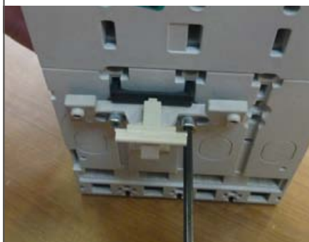
Fix the latch with the two screws supplied (tightening torque 1 N·m).
