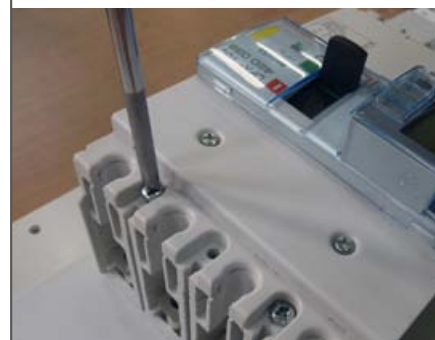
Fix the DPX 3 using the screws supplied with the circuit breaker (tightening torque 1 N·m).
