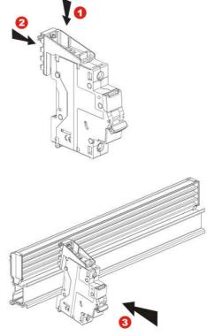
. Connection module 1P+N (cat. n° 4 052 23): No tools required to assembly the connection module to the MCB 1P+N in 1 module with automatic terminals
